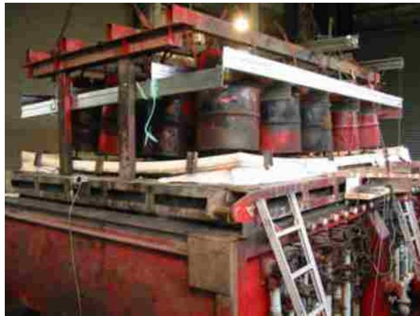
Figure 3-14 Fire testing of slabs (Lim & Wade, 2002)
